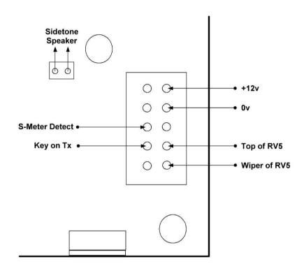
The two holes near electrolytic C5 and R7 are for a sidetone speaker. If you intend to use that facility you can wire it up accordingly.
