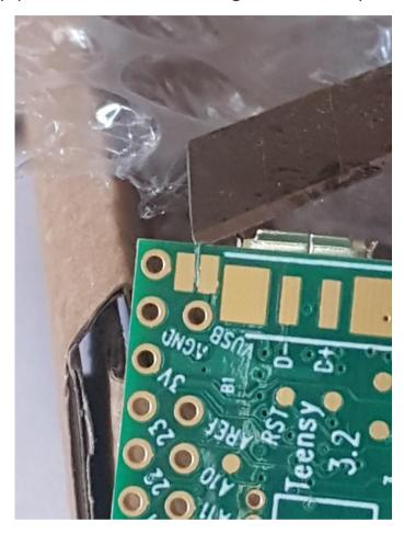
**Note:** Once the track is cut, the Teensy will need external power; the USB will no longer power the PCB.
