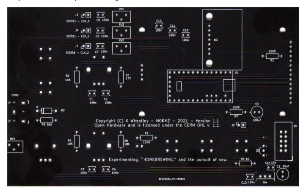
Solder the Teensy (U1) in place on the same side as the Si5351 Break Out Board following the outline on the PCB (see below); you need the main components and the USB socket to be on the top so you can see them. When it comes to soldering it is best to do one pin and check nothing has moved before doing the rest.
